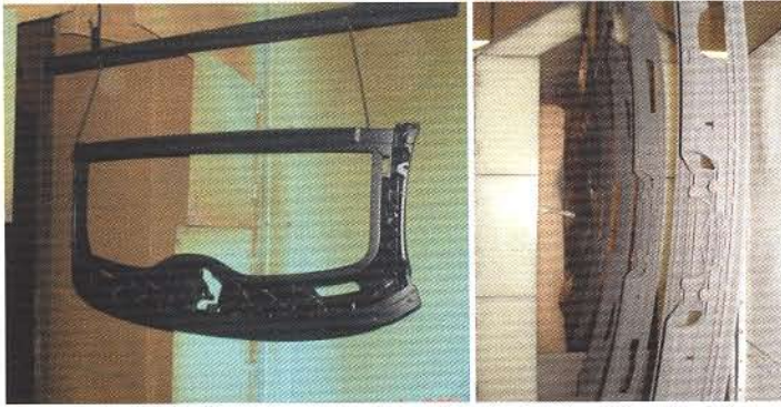
B.L. Downey Co. finishes automotive components on its powder and e-coating lines, including these convertible rooftop components.
